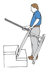
Turn the walker sideways so the crossbar is next to you. Place the first two legs on the step above you. Hold the walker with one hand and the handrail with the other.
